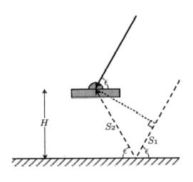
Simple geometry for incidence of a direct and reflected signal
