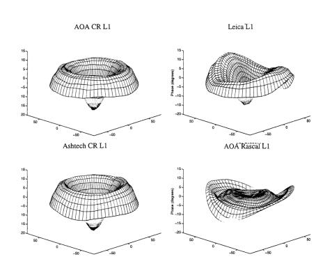
Left: Examples of the antenna phase patterns determined in an anechoic chamber...BUT the actual pattern in the field is affected by the antenna mount
