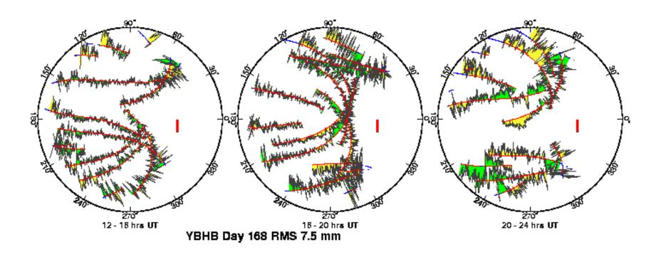
One-way (undifferenced) LC phase residuals projected onto the sky in 4-hr snapshots. Spatially repeatable noise is multipath; time-varying noise is water vapor.
